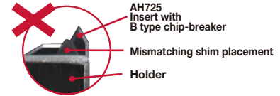
Incorrect insert and shim setting
