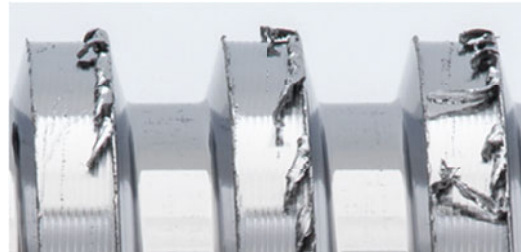
ACME threads without de-burring geometry
